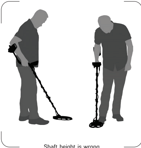
Shaft height is wrong
